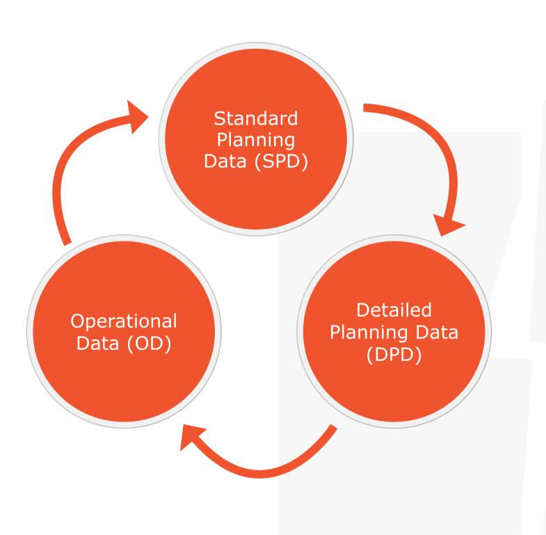
SPD is the data that is required to be supplied by all Users when making application for connection to and/or use of the Disco's Distribution System in order that the DisCo may assess the implications for making the connection
